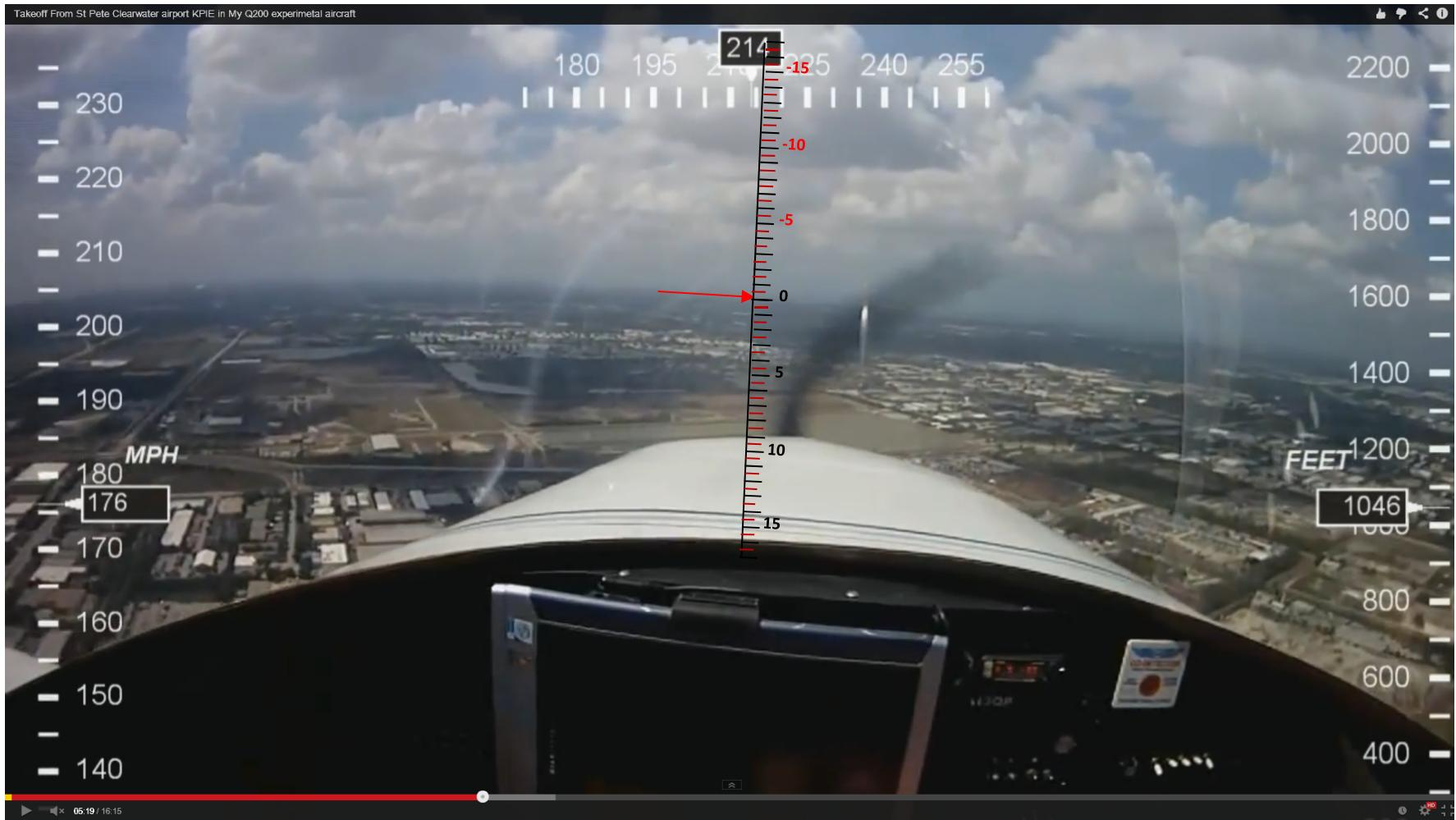
**Figure 12.** View from camera mounted on the seatback bulkhead. The vertical scale in the middle of the image is an angular scale that is calibrated to fixed points on the aircraft. The other scales (from Dashware) are: altitude (right), speed (left), and heading (top). This view is level, over 1000 feet MSL altitude and at max cruise (176 mph) at an alpha of -0.2 degrees. No confirmation of elevator deflection is possible at this point in flight.
