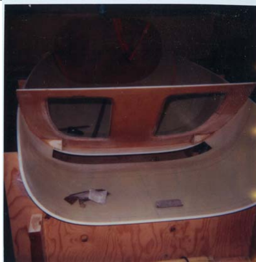
Seat back bulkhead installed w/ micro 1/2/86 Seat lug boxes cut and fit and floxed in seat back bulkhead, 1/3/86
