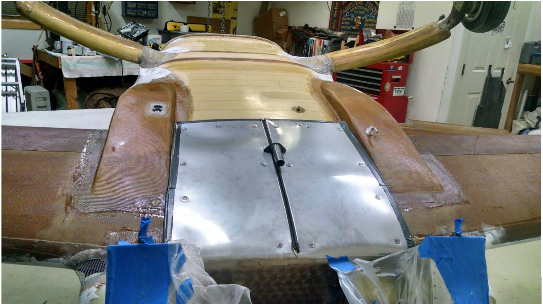
View of stainless steel heat shielding in place, just prior to fuselage filling and priming. Leading edge of stainless sheet fits in behind stainless firewall to completely protect leading edge of canard from any engine heat. October, 2017
