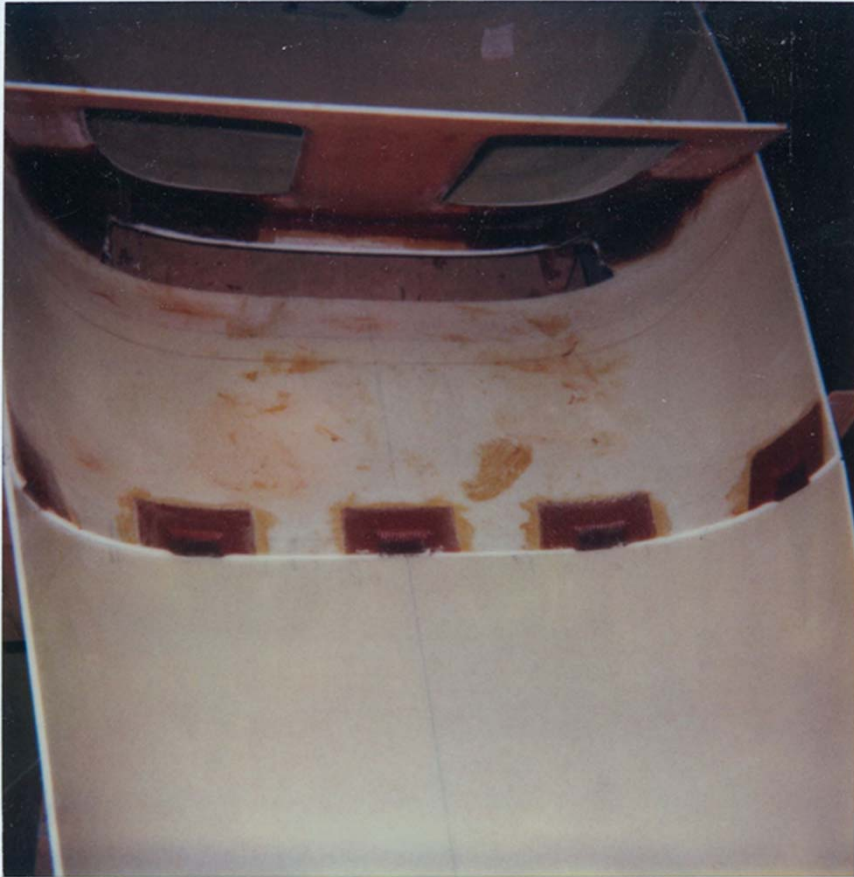
Glassed attach points shown with rear fuselage shell in place. 1/6/86
