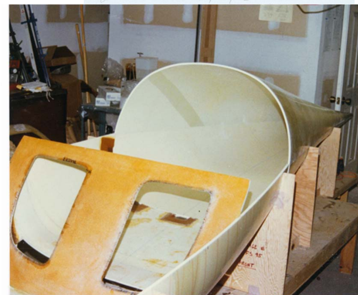
Detail gear aligned through cutout in fuselage - verified square to BL 00 12/31/85
