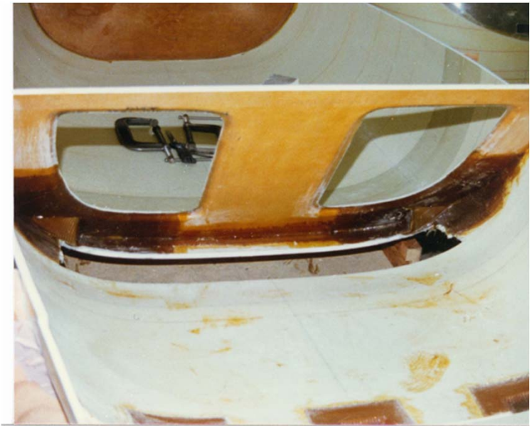
REAR GEAR ATTACH - BULKHEAD MICRO'ED IN PLACE AWAITING FUSELAGE WRAP (2 BID) and 10 ply wrap around layups 12/4/86
