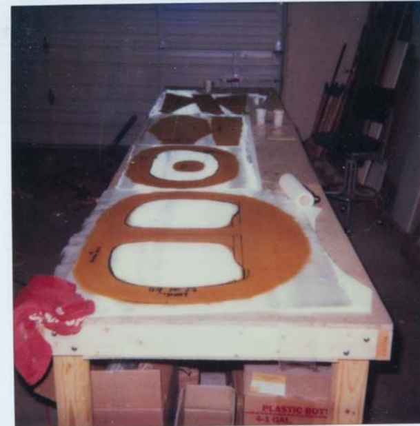
GLASSED BUT UNTRIMMED BULKHEAD + CONSOLE PIECES 2/24/85
