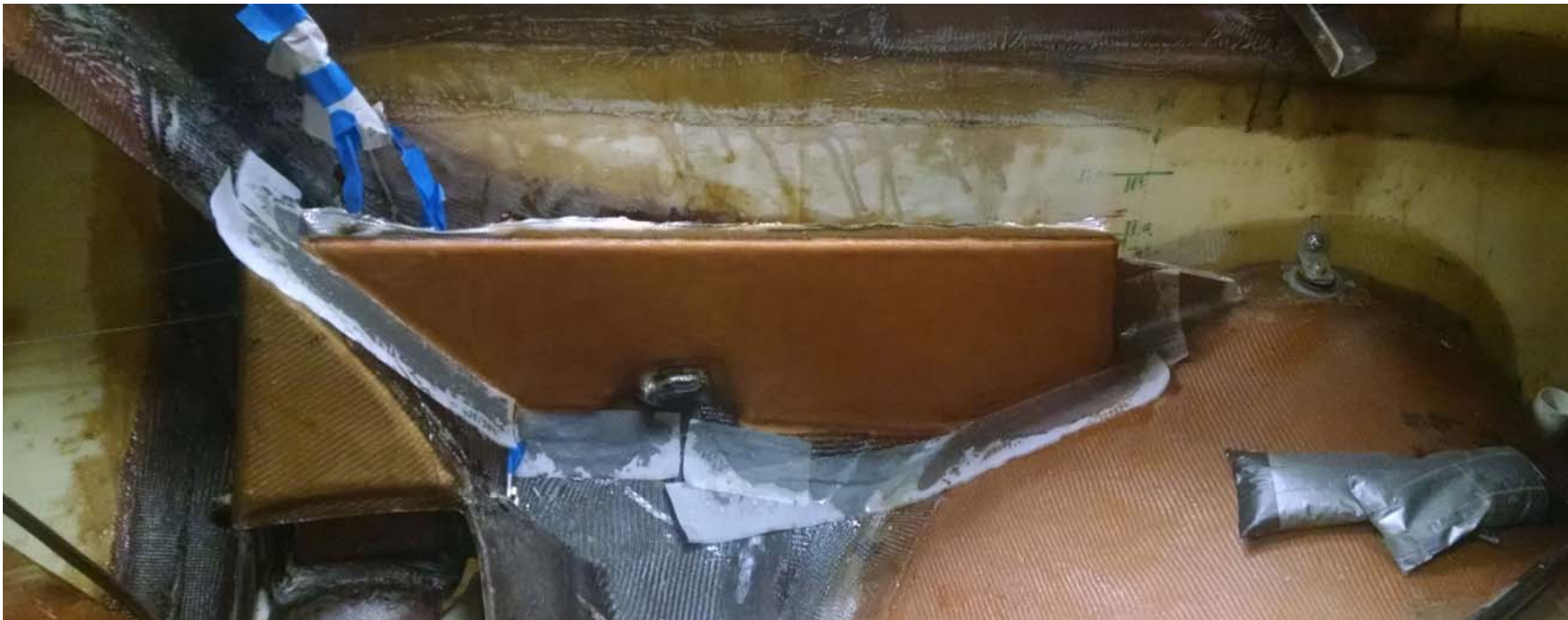
Glass lower console panel to main tank, fuselage and seatback with 2 BID.
