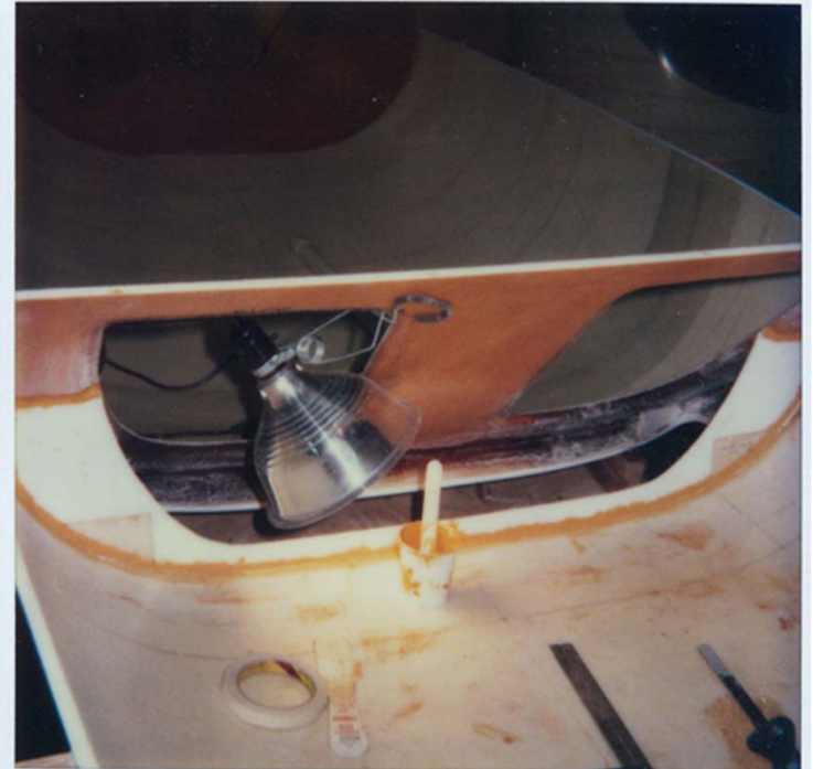
REAR GEAR ATTACH - BULKHEAD MICRO'ED IN PLACE AWAITING FUSELAGE WRAP (2 BID) and 10 ply wrap around layups 12/4/86
