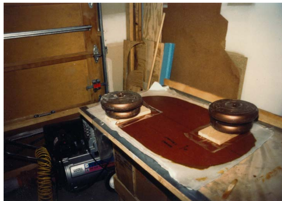
Firewall cut from plywood and fit to fuselage, then glassed (both sides) on flat table. Firewall positioned and floxed in place per plans. Work and layups verified by Jay Scheevel –Jan. 1986
