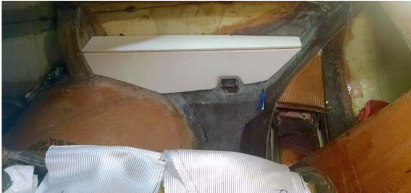
Trim and fit previously made side consoles. June, 2016
