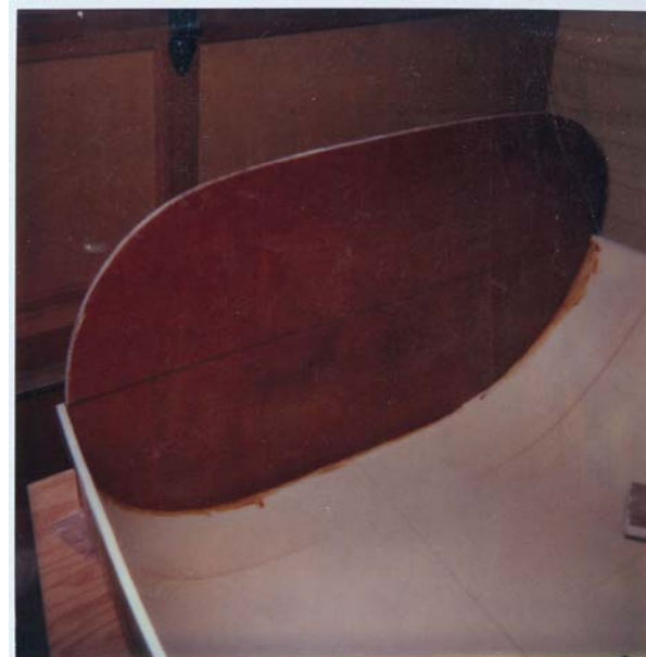
Fire wall installed w/ flox - to be glassed later 1/3/86
