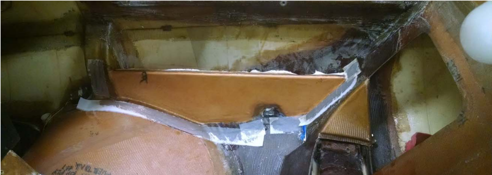
Glass lower console panel to main tank, fuselage and seatback with 2 BID.
