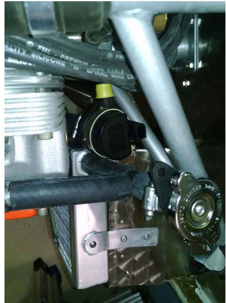
Radiator, water pump and plumbing detail view from top is shown at right. January, 2016
