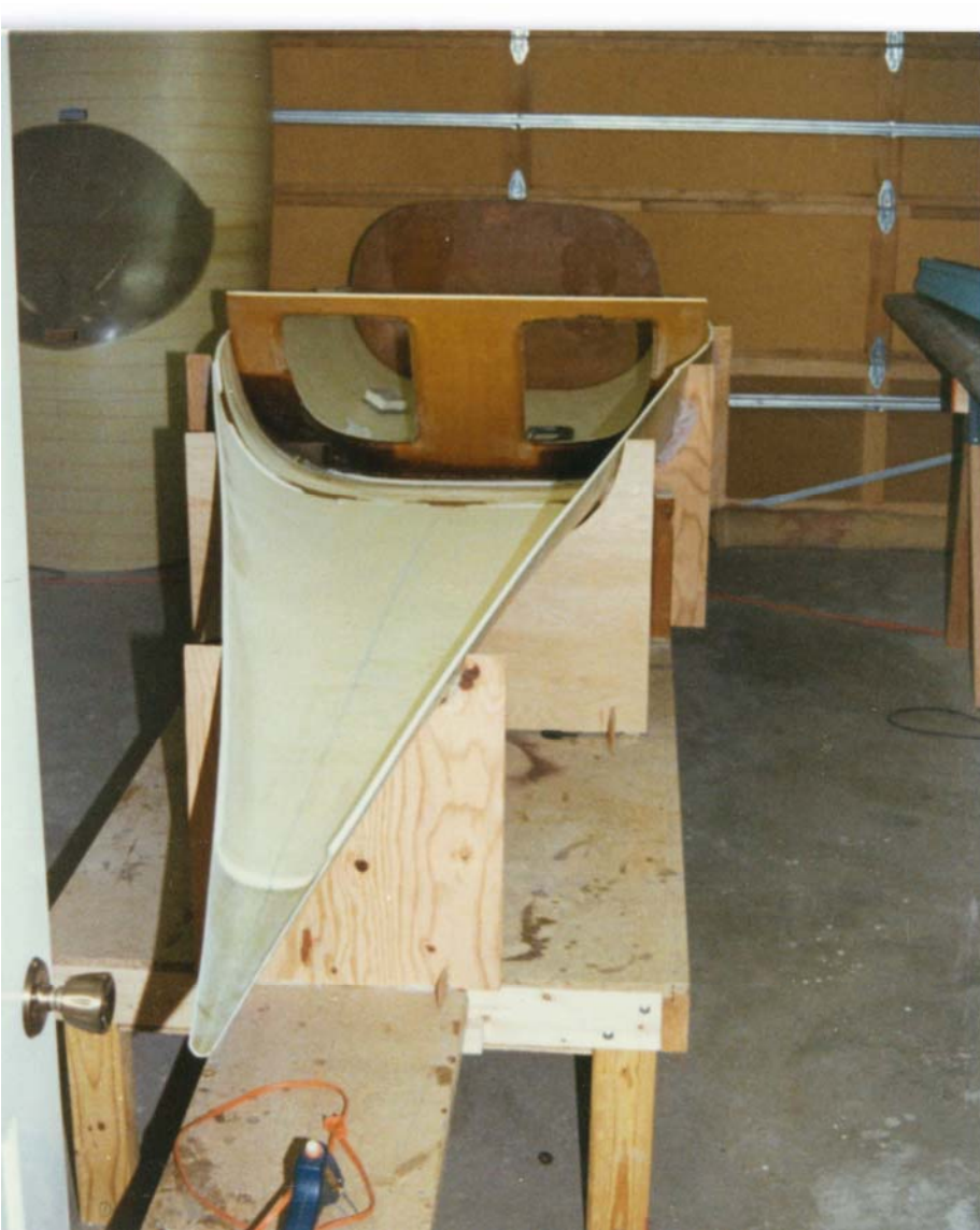
Firewall cut from plywood and fit to fuselage, then glassed (both sides) on flat table. Firewall positioned and floxed in place per plans. Work and layups verified by Jay Scheevel –Jan. 1986
