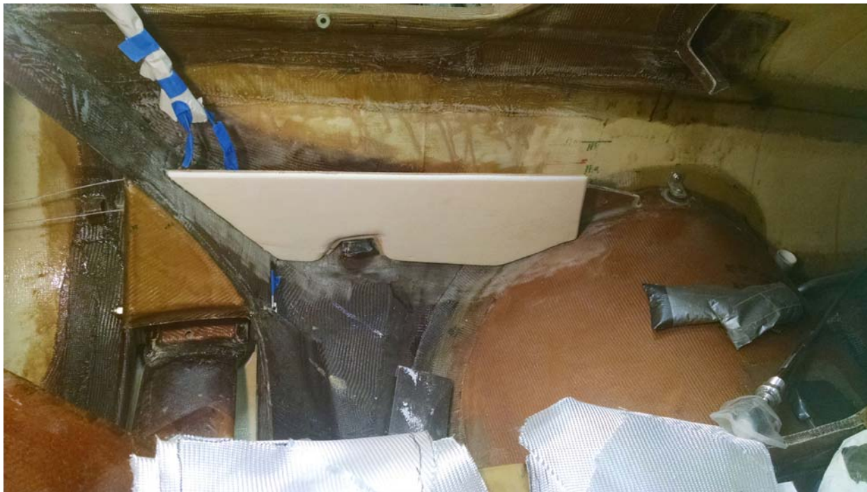
Trim and fit previously made side consoles. June, 2016
