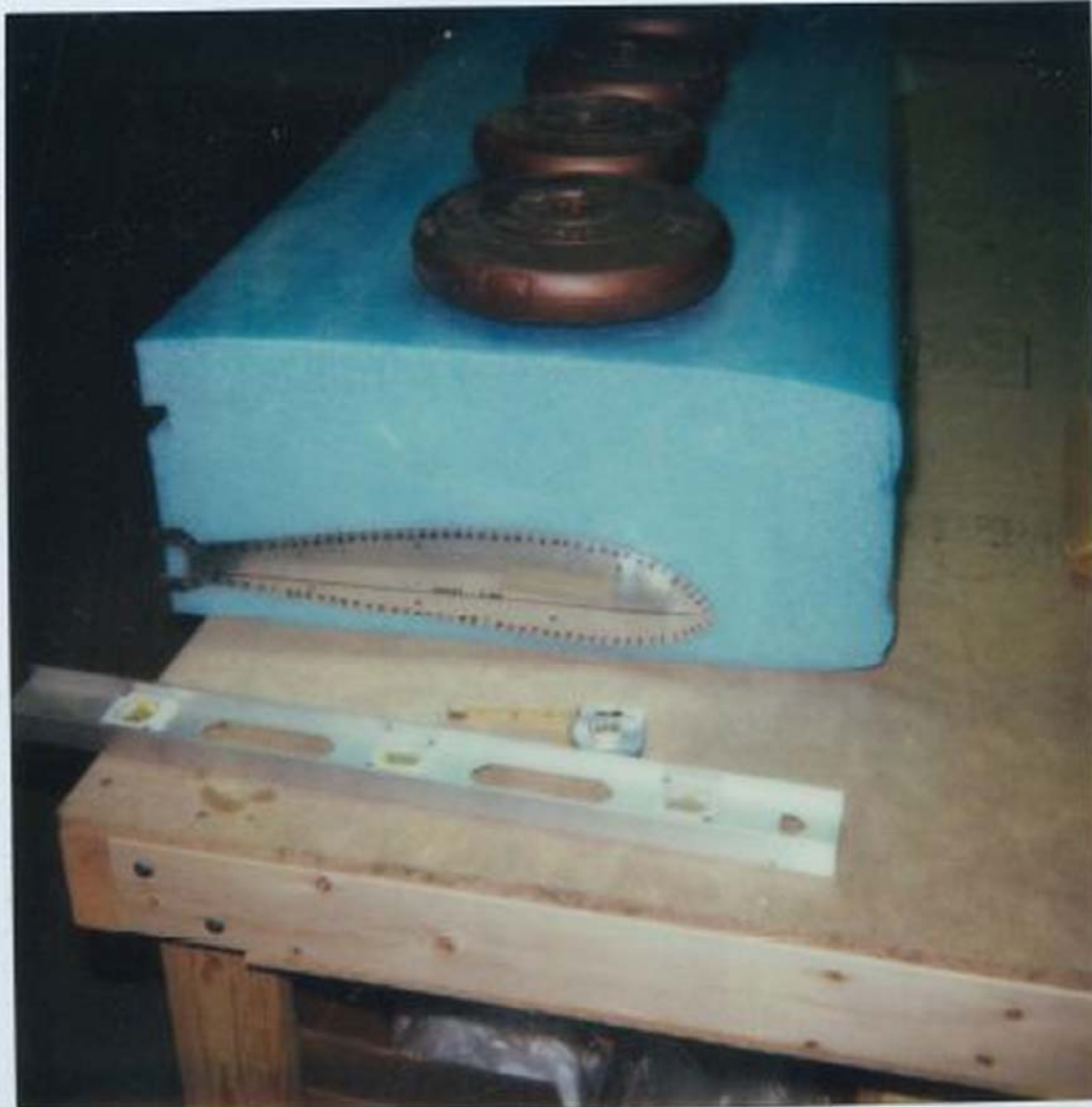
TEMPLATE AND FOAM BLOCK FOR HOT WIRE CUTTING OF MAIN WING. 11/13/84
