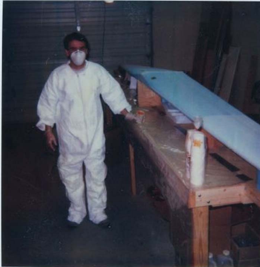
WAYNE IN ANTI-EPOXY OUTFIT W/ WING-CORES READY TO GLASS 2/16/85 SHOULDER HARNESS SUPPORTS ARE FLOXED IN PLACE
