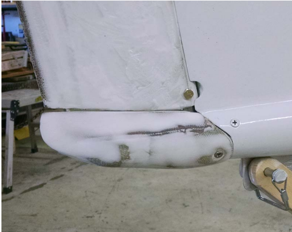
Rudder assembly with tailcone fairing fastened into position. Spindle is entirely within fairing. Verify motion and free travel. November, 2017
