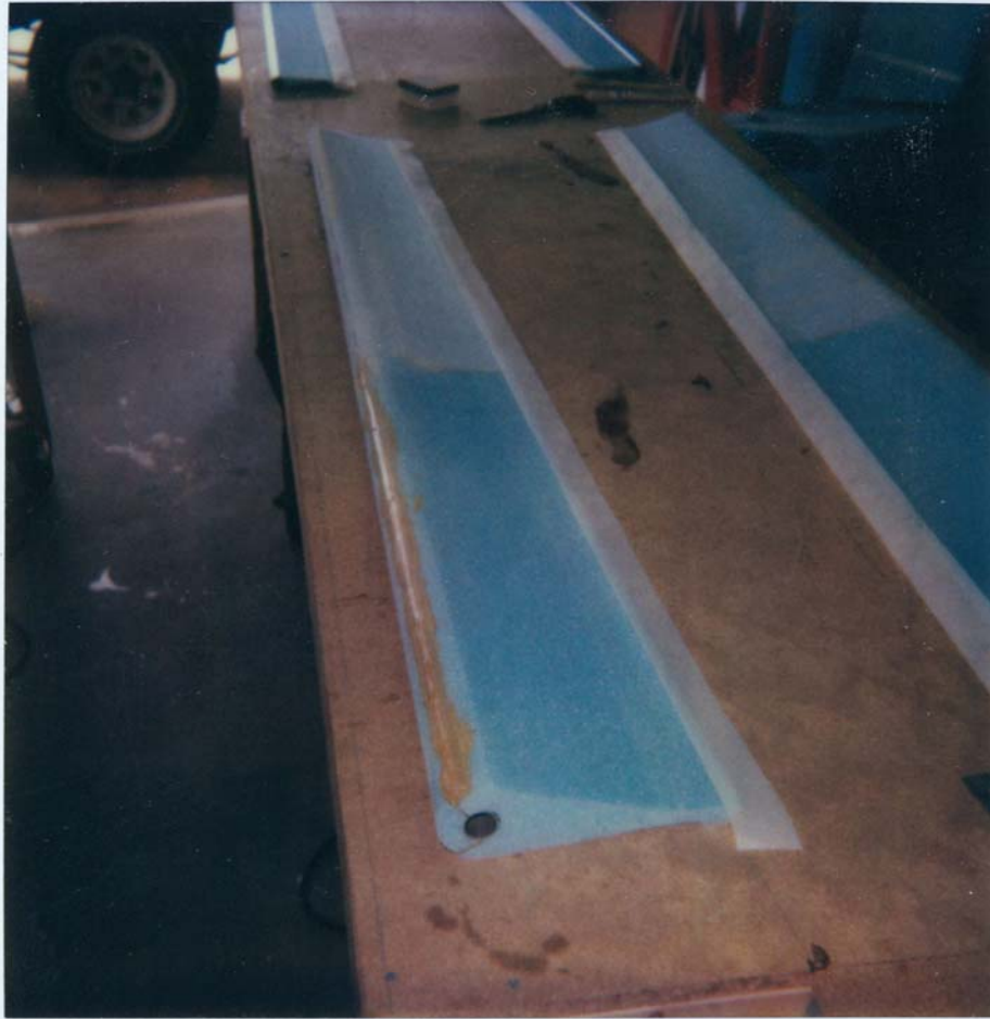
tops of elevator core microed and prepped for glossing 8/11/85
