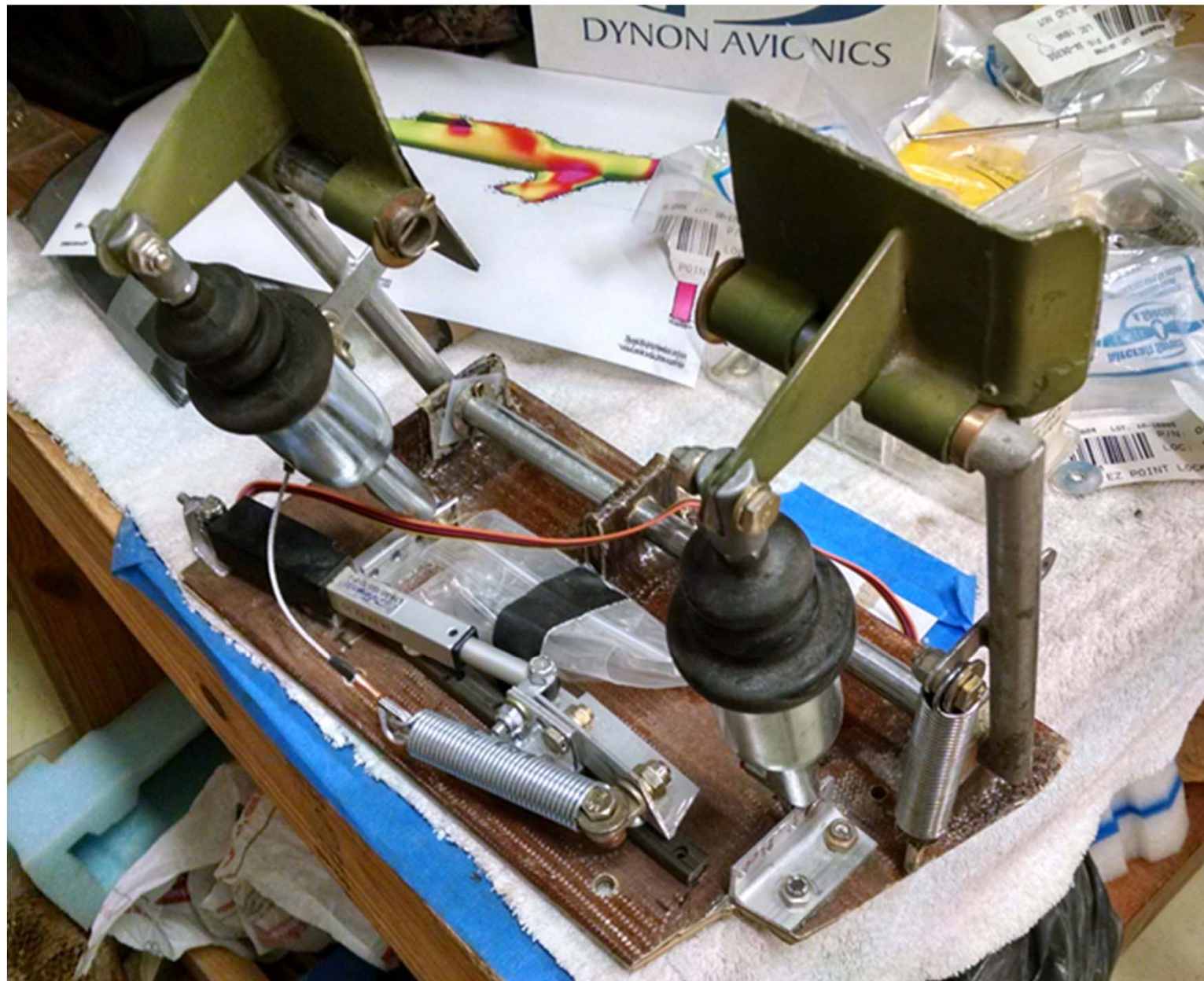
Fitting rudder pedals to brake cylinders and testing clearance and range of motion and security on brake platform.
