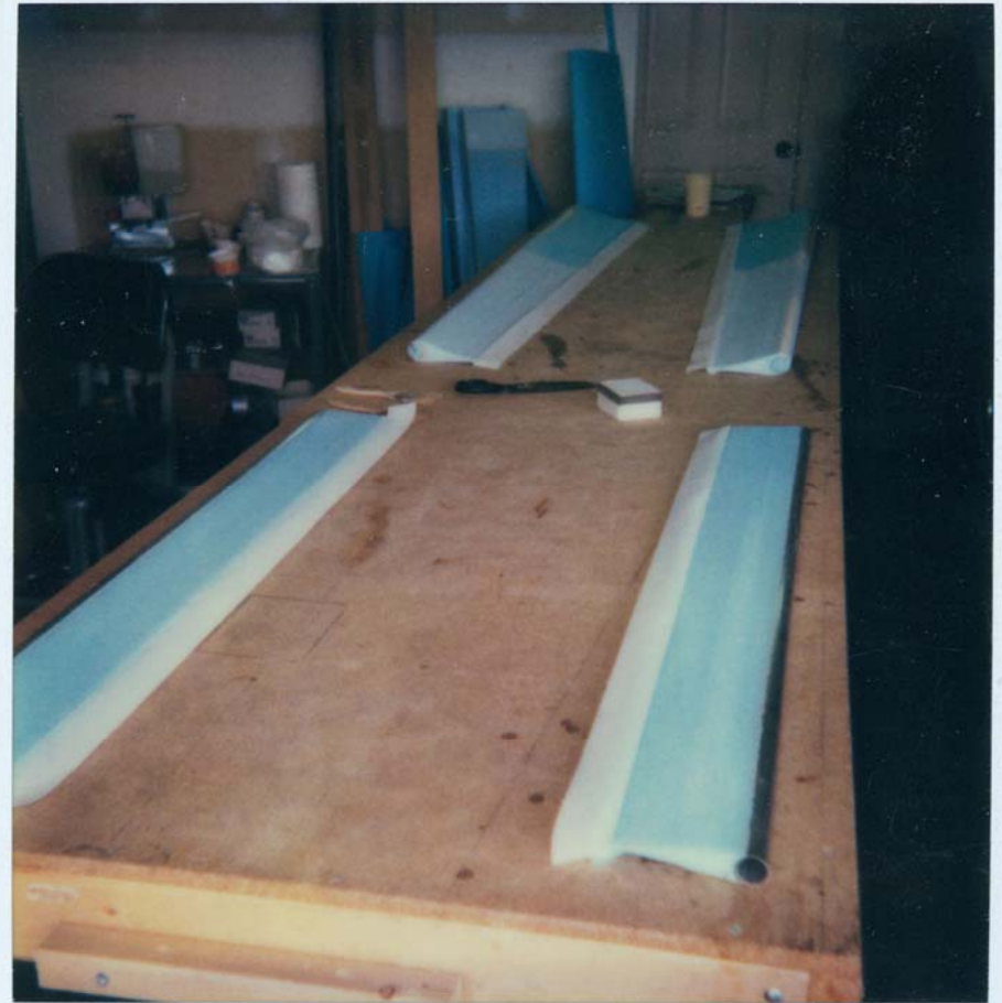
Tops of elevator and aileron cores prepped for glossing - leading and trailing edges bonded to flat surface 8/11/85
