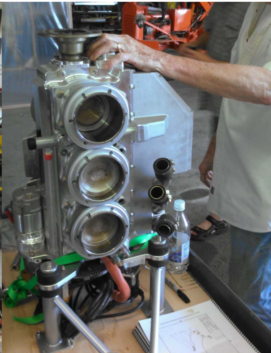
Good friend and A.I., Gerry Miller assisting and reviewing replacement of air cooled heads and replacement with Rotec water cooled heads per Rotec instructions.
