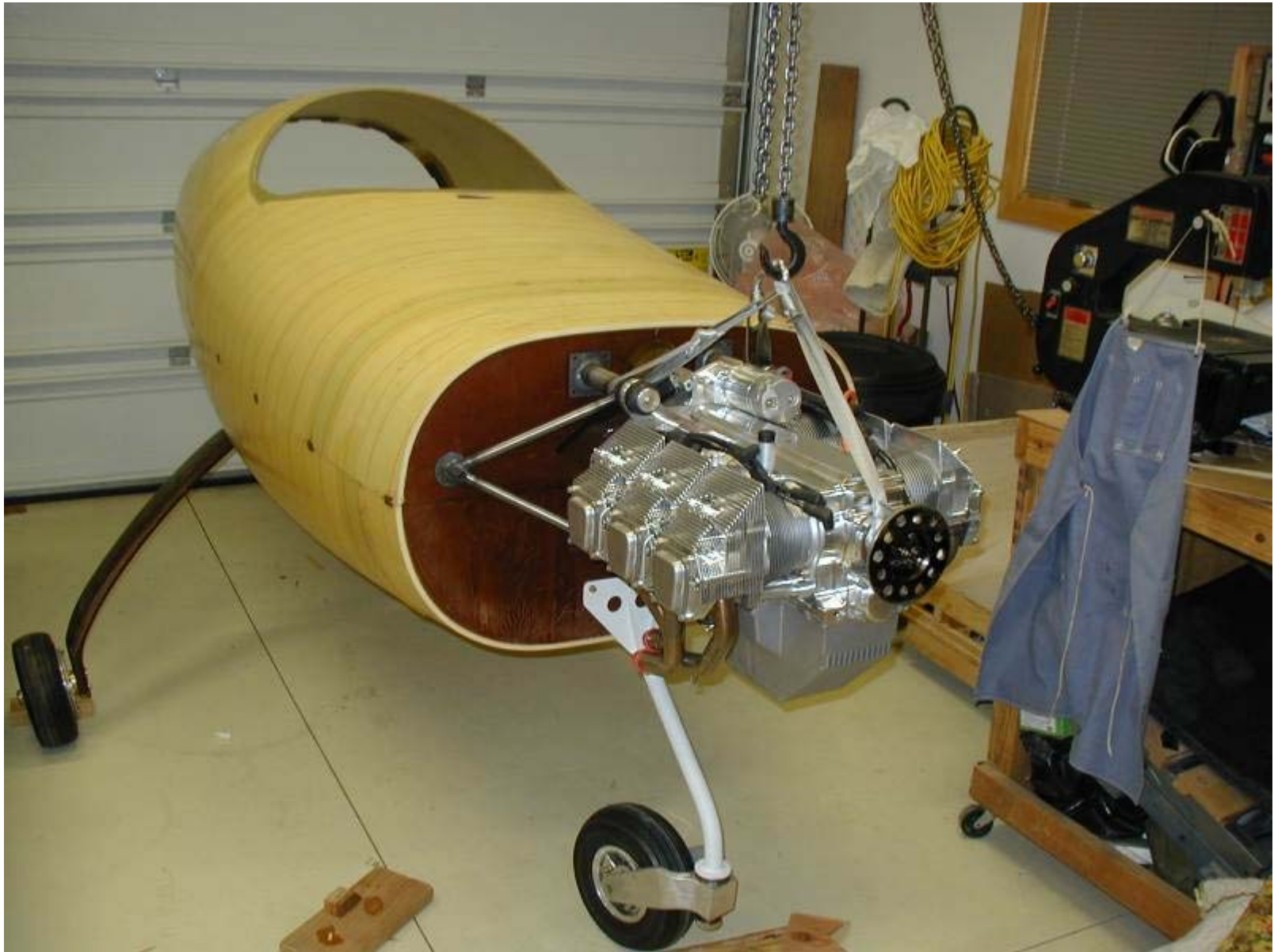
Test fit new Jabiru 3300 engine and Paul Spackman style engine mount to the firewall, adjusting thrustline to match O-200 from Q-200 plans.
