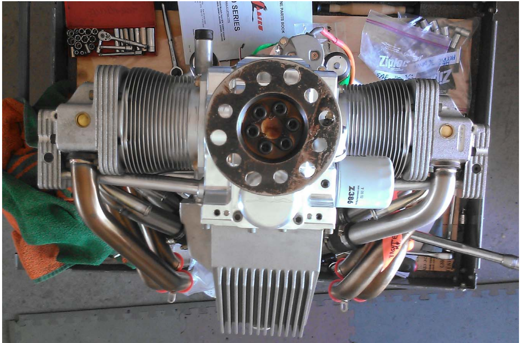
Reassembled engine with new water cooled heads in place.
