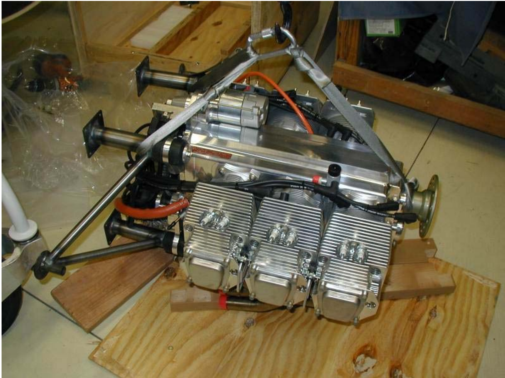
Jabiru J3300A, SN 1891 after uncrating and fitting to Paul Spackman style engine mount.
