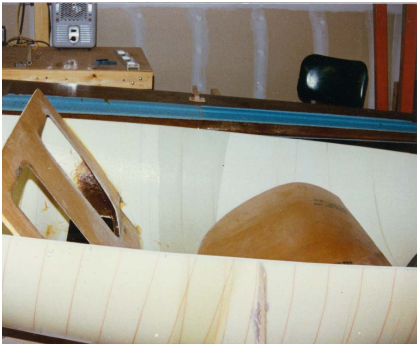
Trim and fit main tank to the contour of the fuselage in proper position in front of seat back bulkhead. December 1985
