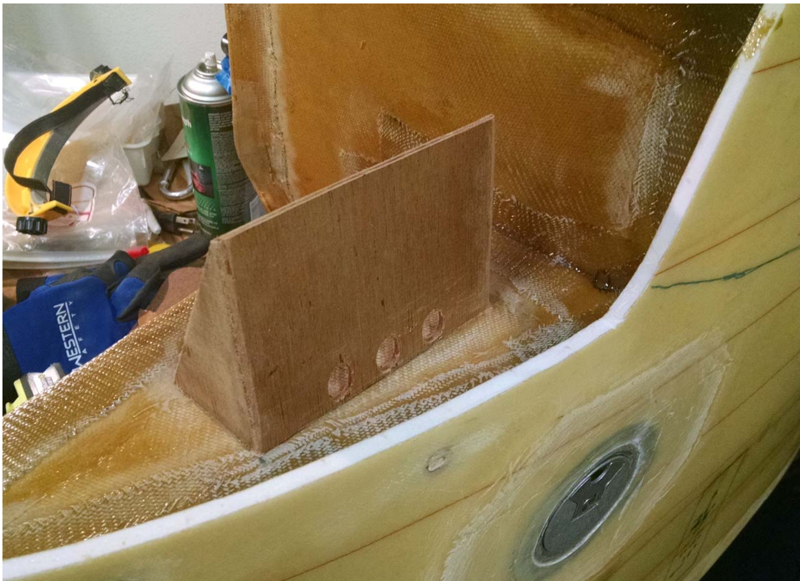
Install mahogany shelf on rear panel of header tank to hold the ADHRS sensor package for Skyview system avionics package. February 2016
