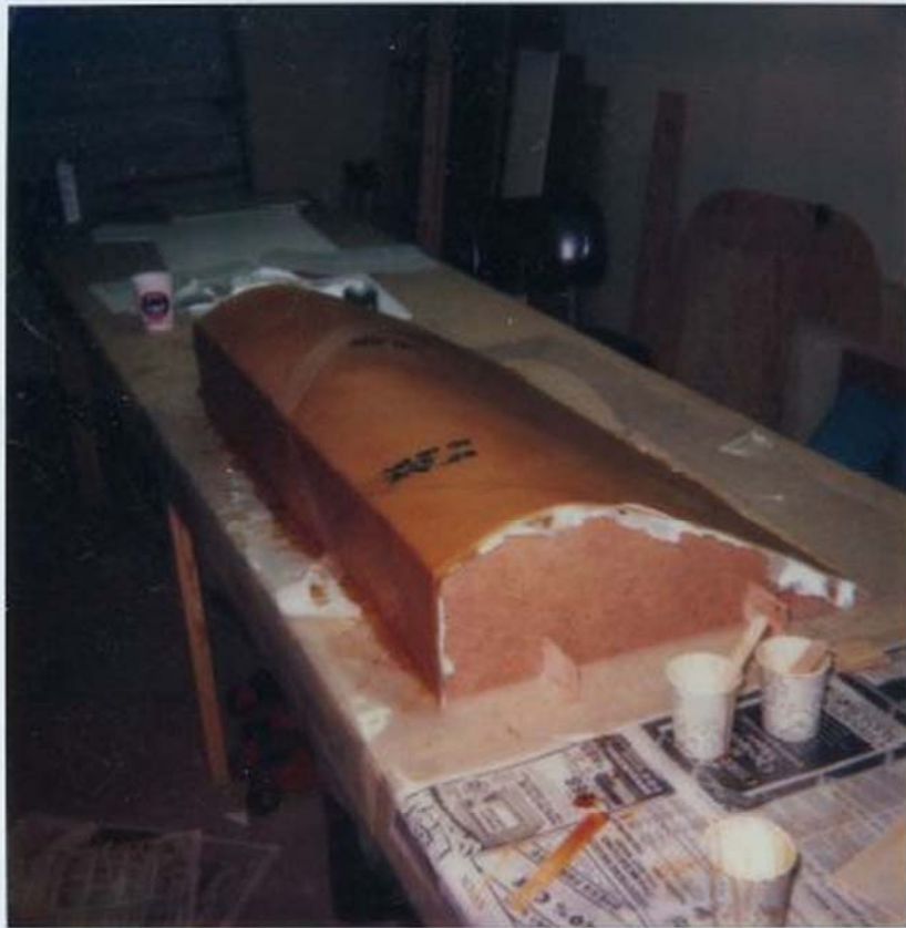
COMPLETED 2 PLIES OF BIDIRECTIONAL CLOTH ON FUEL TANK 11/25/84
