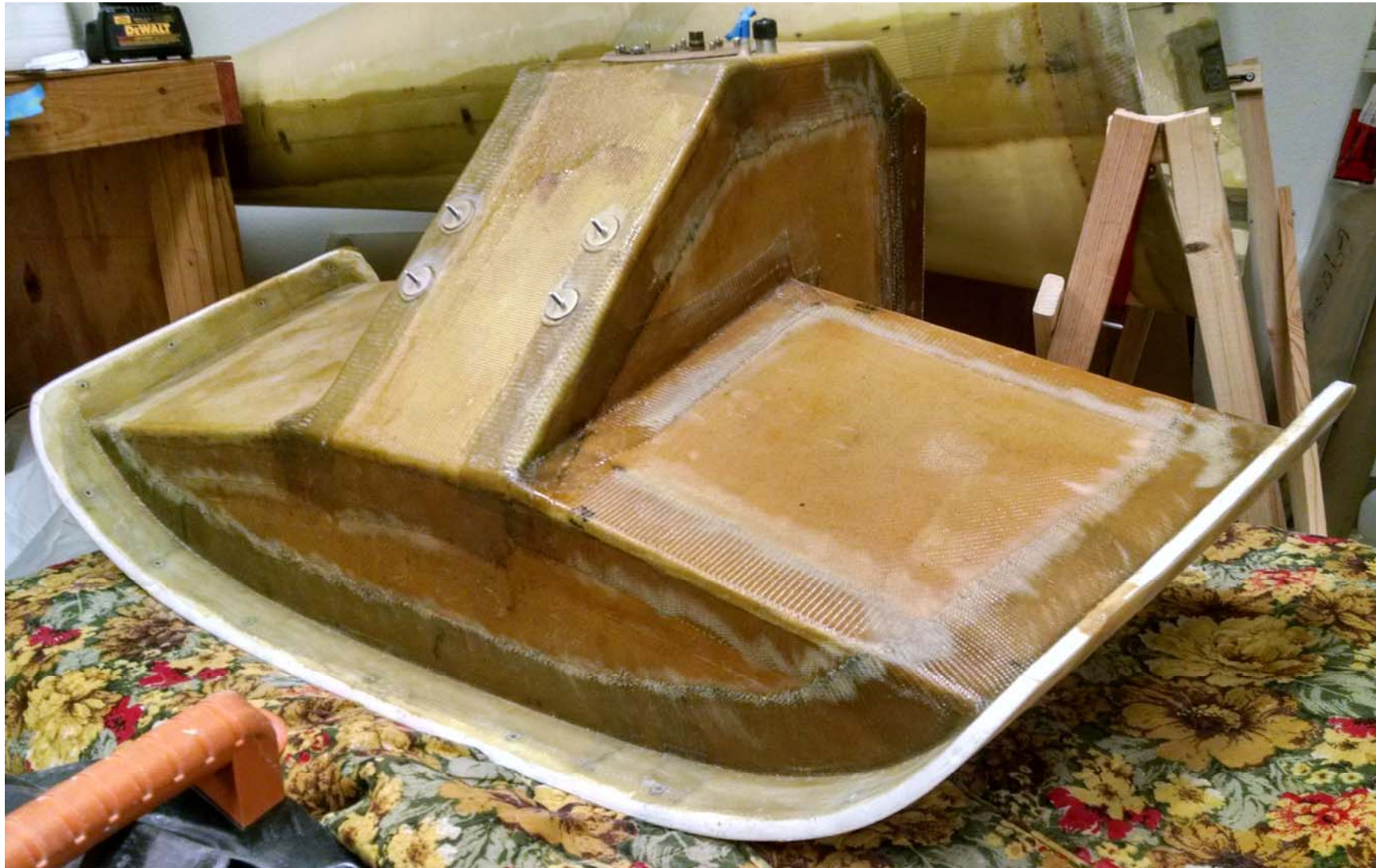
Install mounting hardware for Skyview EMS box on sloping front of header tank. June 2016
