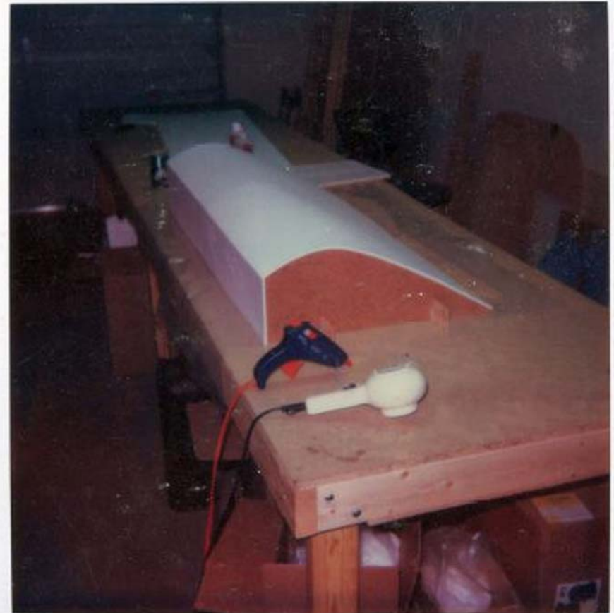
FUEL TANK FOAM FORMED OVER TEMPLATE READY FOR GLASSING 11/24/84
