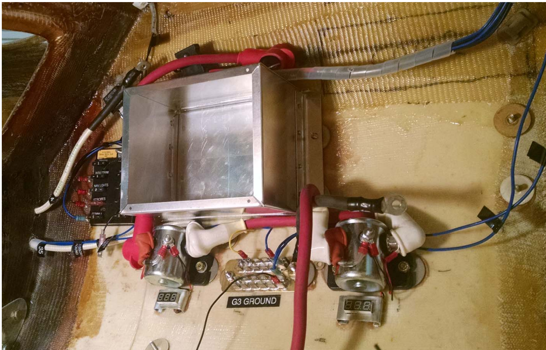
View of Main battery box fitted into position on mount brackets and 10-32 EX-point pedestal mounts. Also note position of G3 ground block and both Main and Aux battery contactors.
