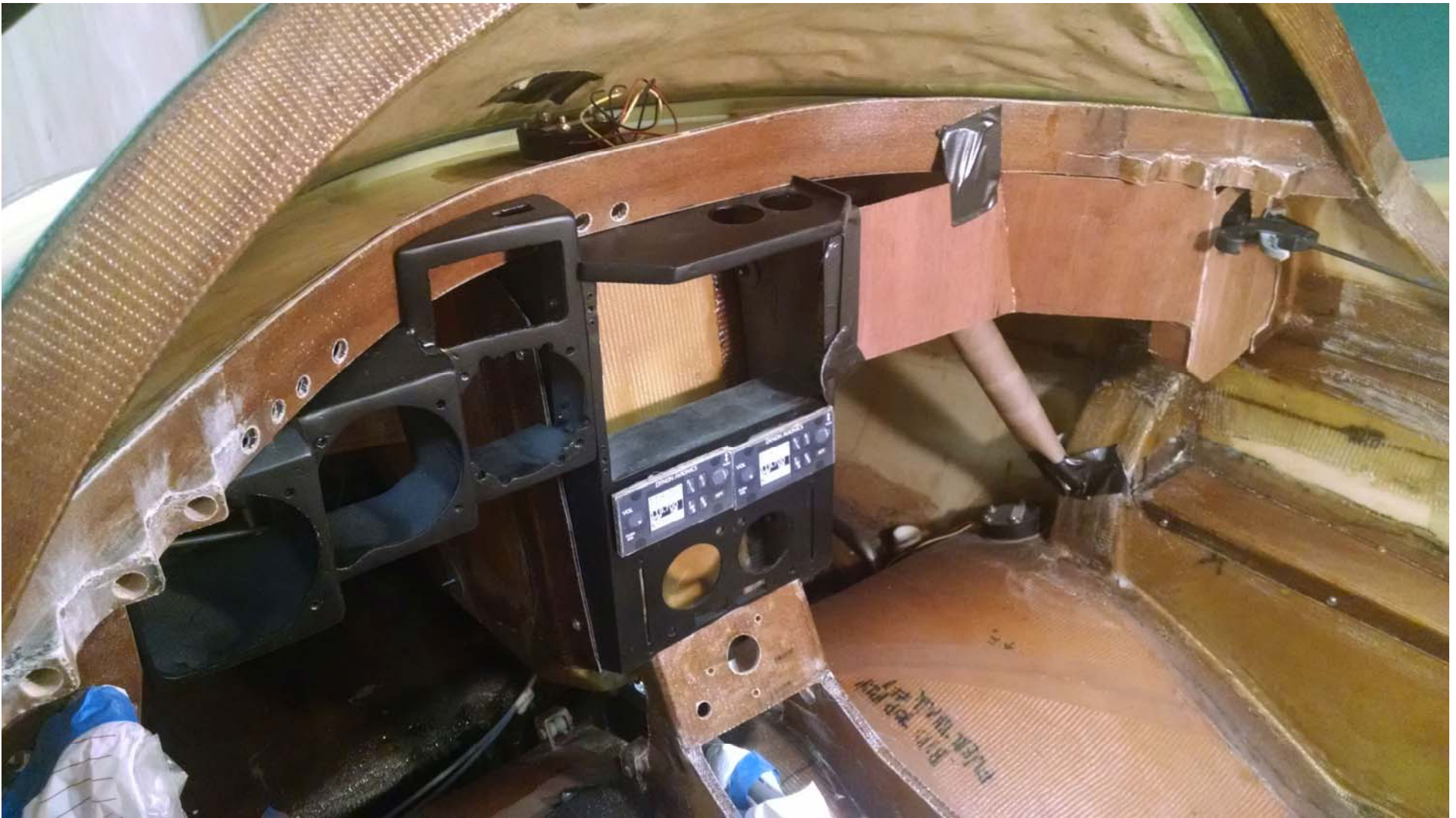
Passenger side consoles laid out, designed and constructed of 1/16" plywood. Right console support anchor designed and glassed to fuselage side. July 2016
