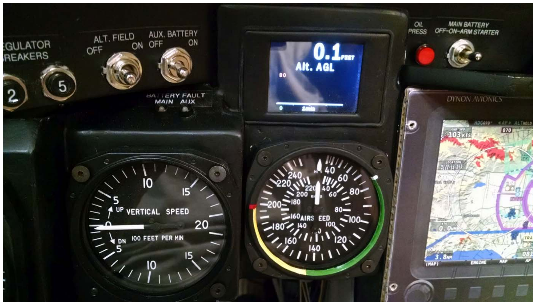
Final layout and test of laser altimeter. Note position on panel relative to other instruments. The EFIS in this photo is a cardboard mock-up.
