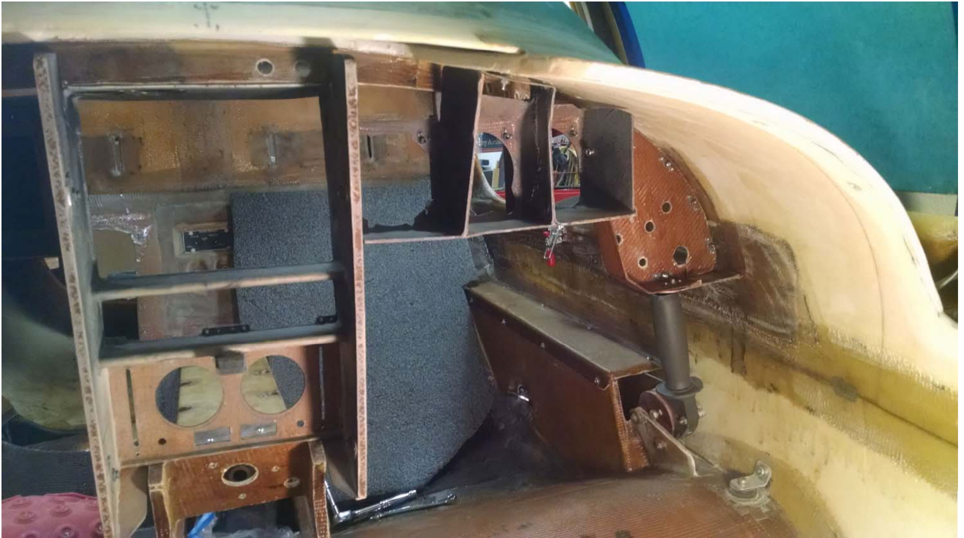
View of the pilot's side panel components from behind the panel. Engine control panel on the right, instrument cluster to the left of that and center console to the left of than. Gray stick on right, below the engine control console is the reflexor control stick. January, 2017
