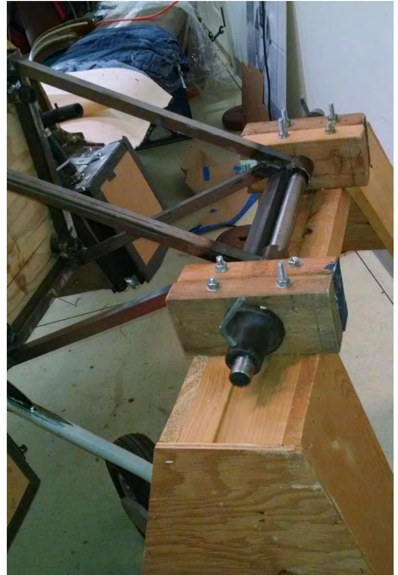
Build support/pivot assembly for supporting fuselage with nose wheel removed for filling, priming and painting. July 2017.
