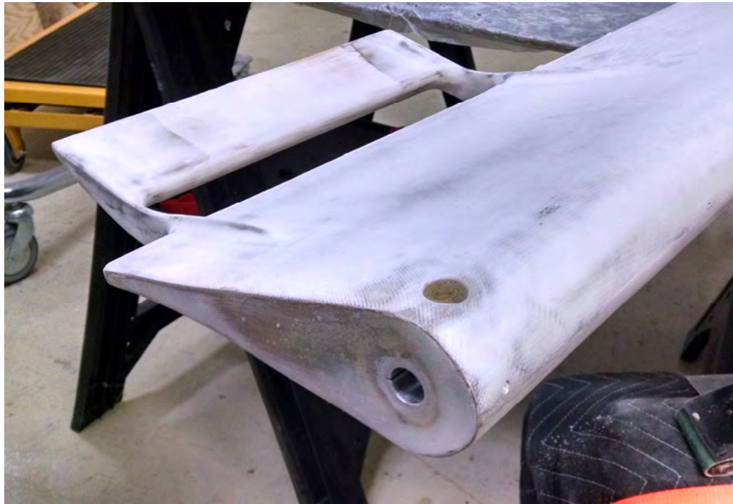
Sand and contour elevators and sparrow strainers and ends of control surfaces. November 2017
