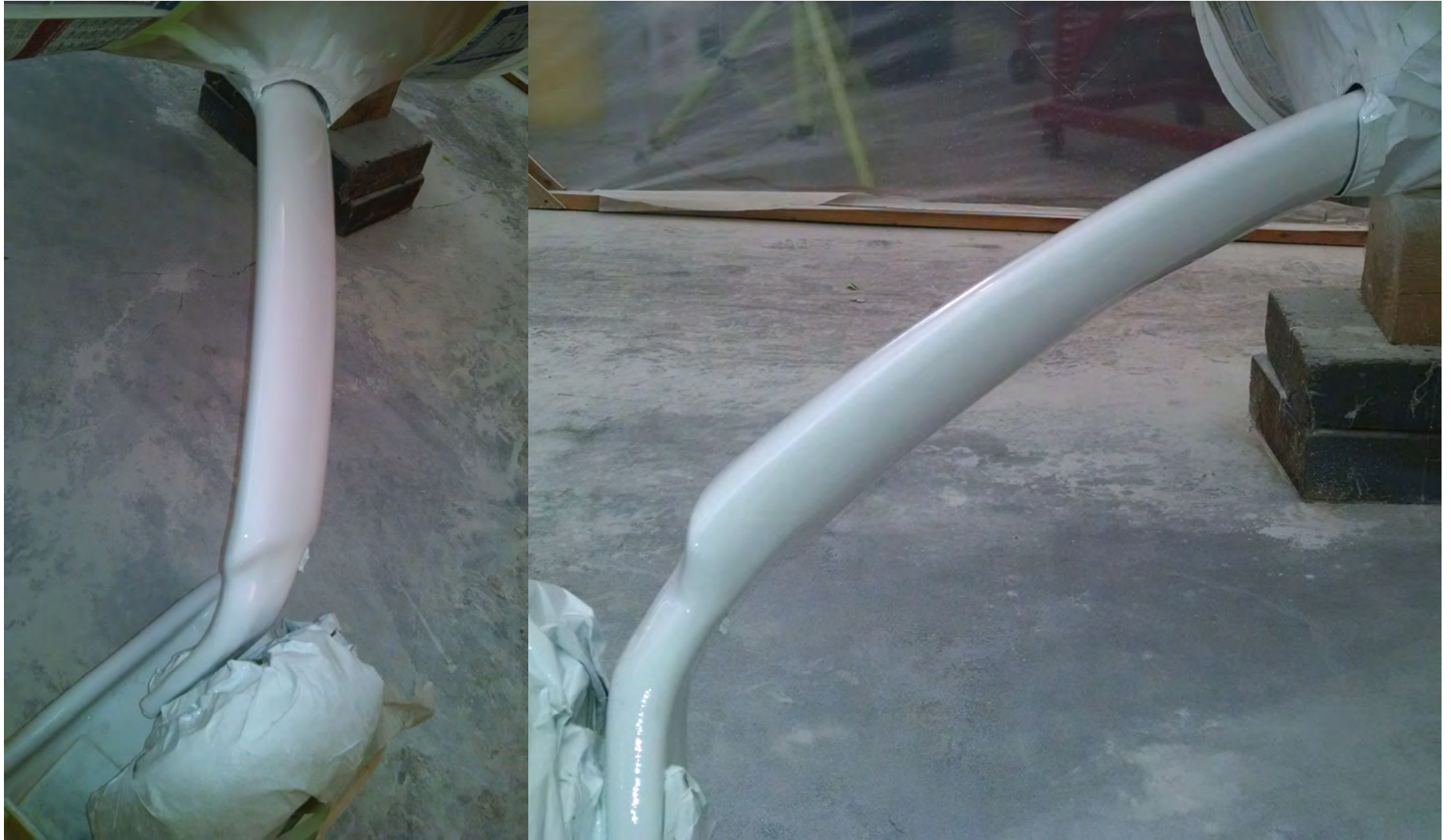
Final sand and spray final color single stage white on gear legs. January 2017
