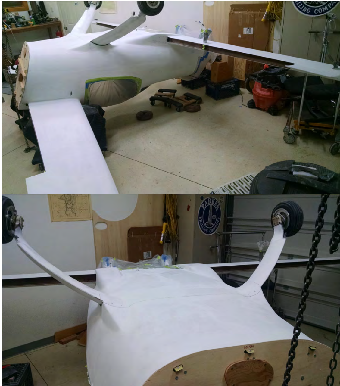
Apply fill primer on lower part of fuselage. October 2017
