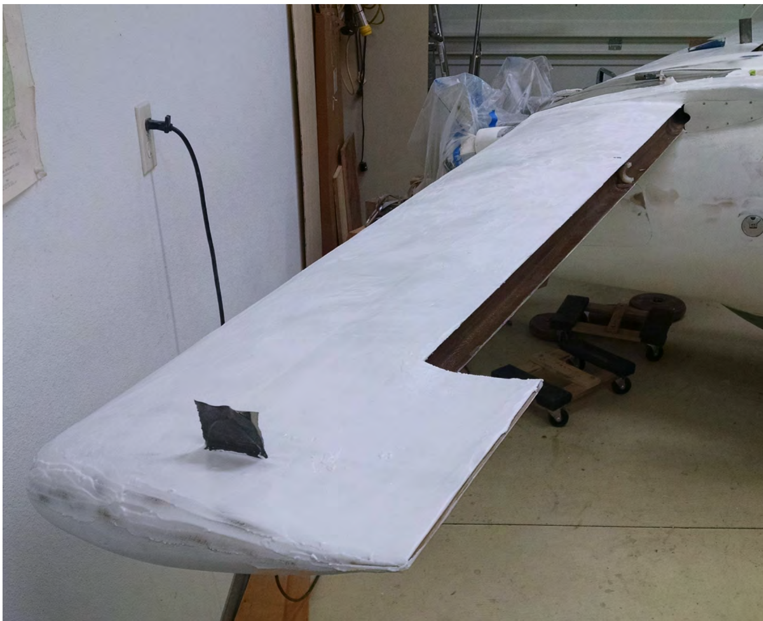
Apply micro to bottom and tip of the right canard. October 2017
