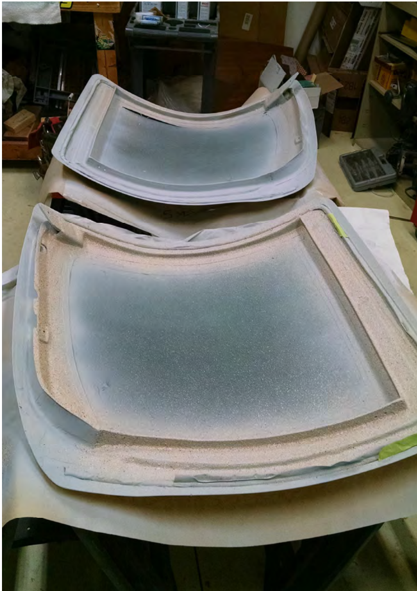
Mask, prime and apply textured paint coats to cockpit door frames. November 2017.
