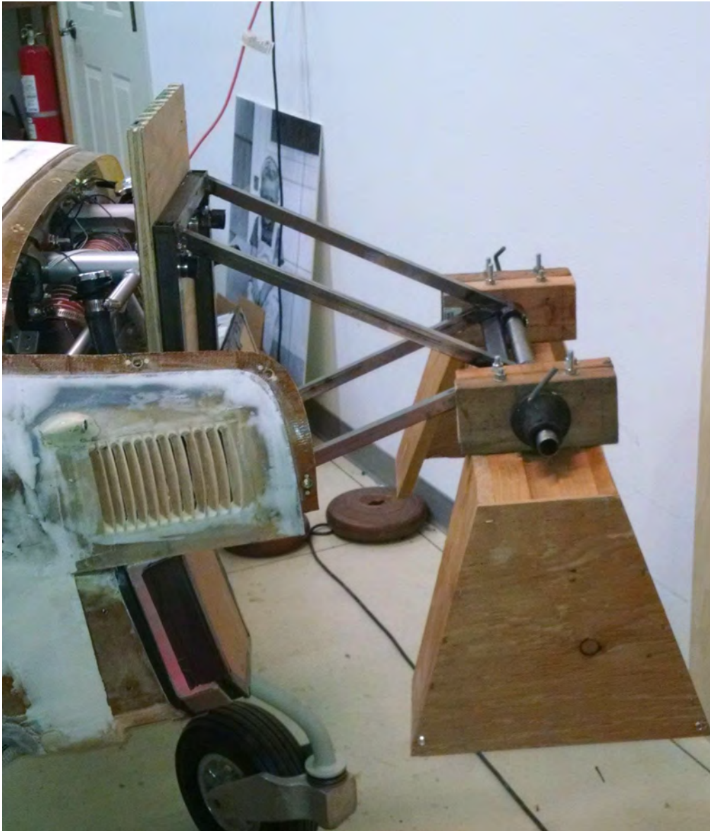
Build support/pivot assembly for supporting fuselage with nose wheel removed for filling, priming and painting. July 2017.
