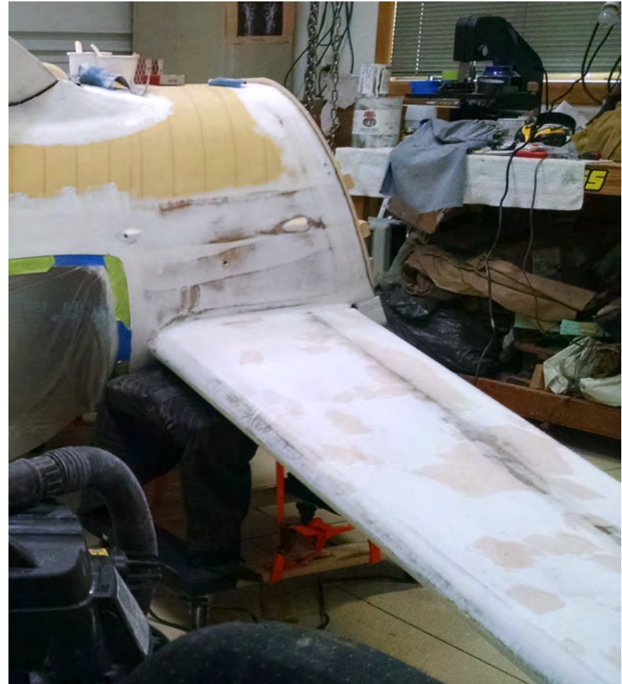
Pinhole filling with West System epoxy.
