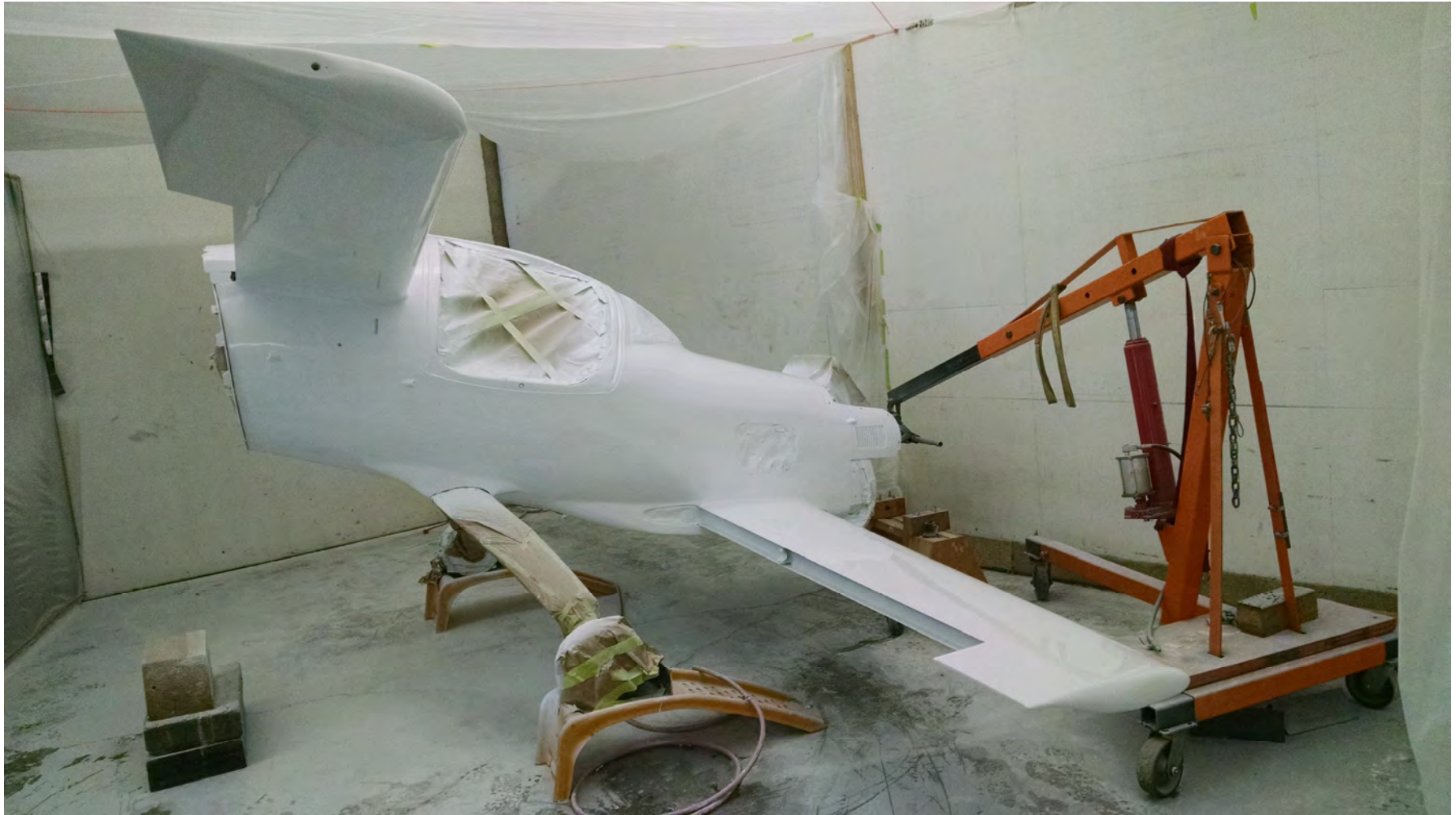
Final single stage color coat is painted over entire airframe. January 2017
