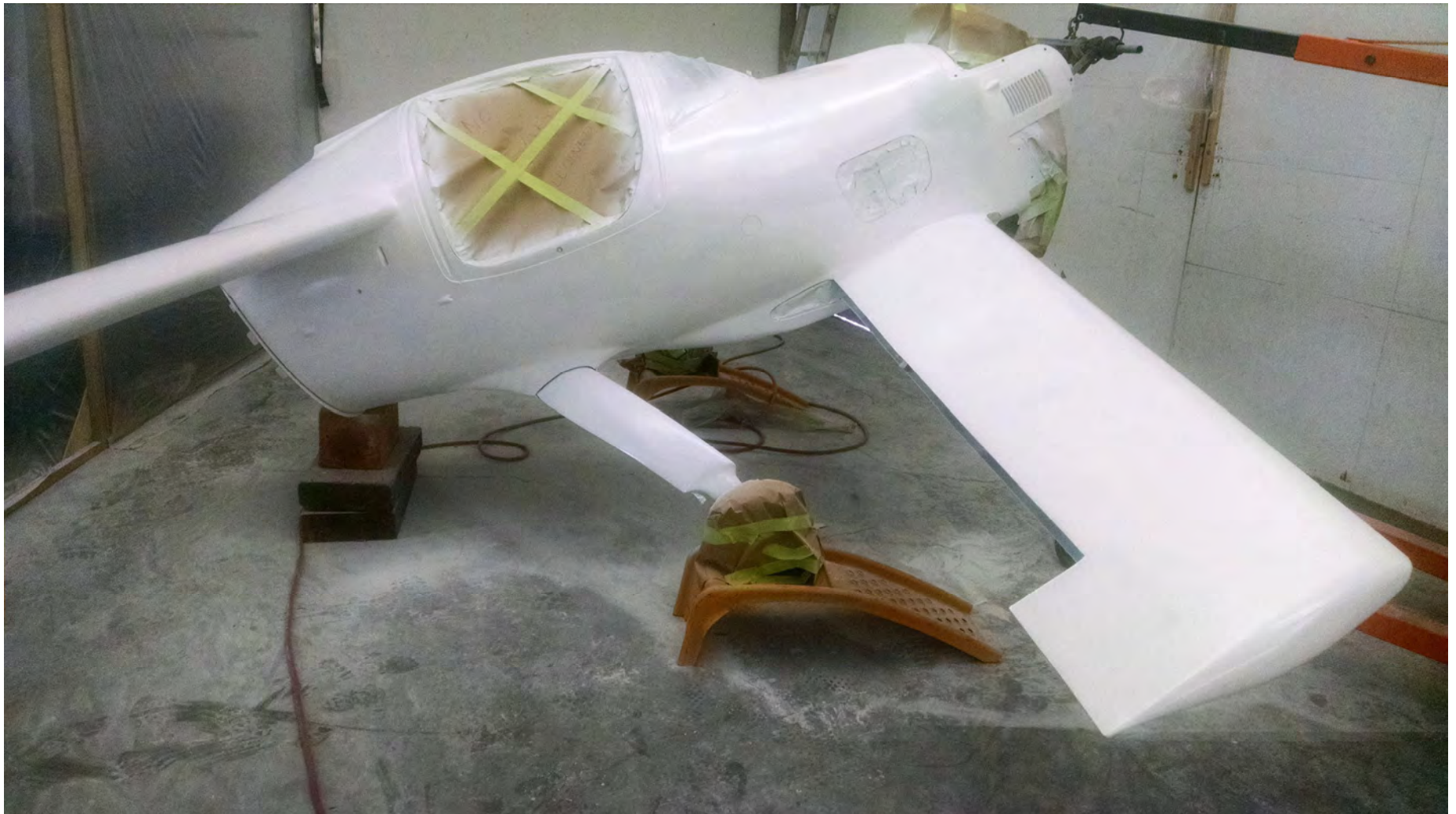
First epoxy spray primer followed by local filling and contouring. December 2017.
