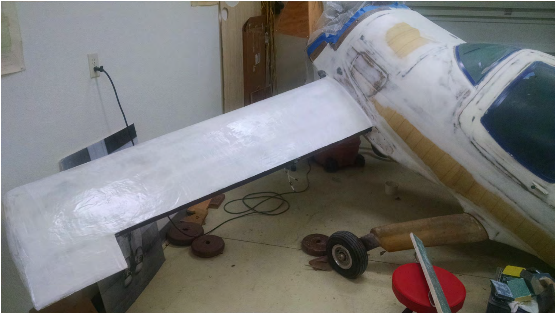
Tilt fuselage back and apply micro fill to upper left canard. September 2017
