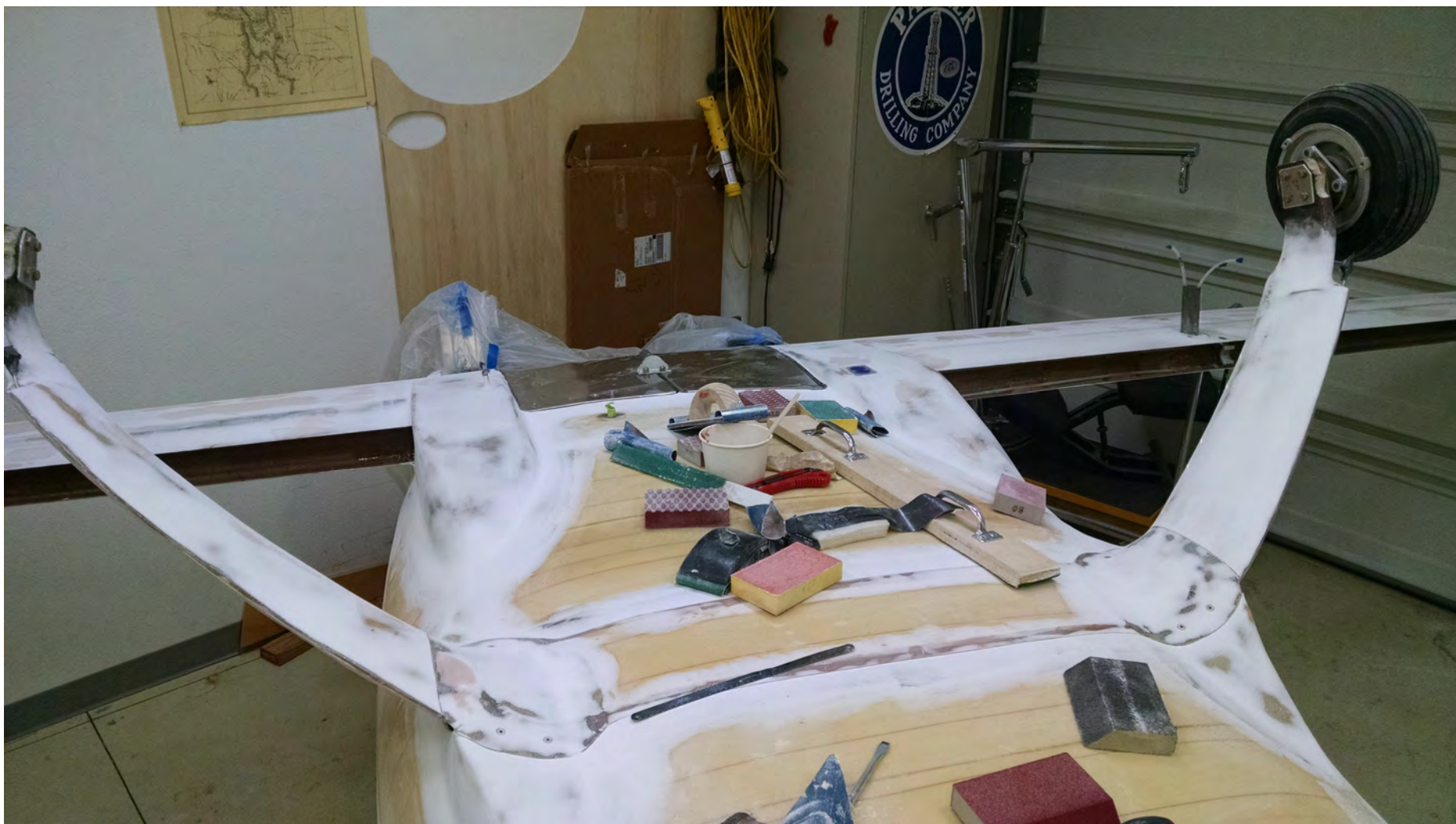
Sand and contour shape in landing gear legs, strakes and fairings. October 2017
