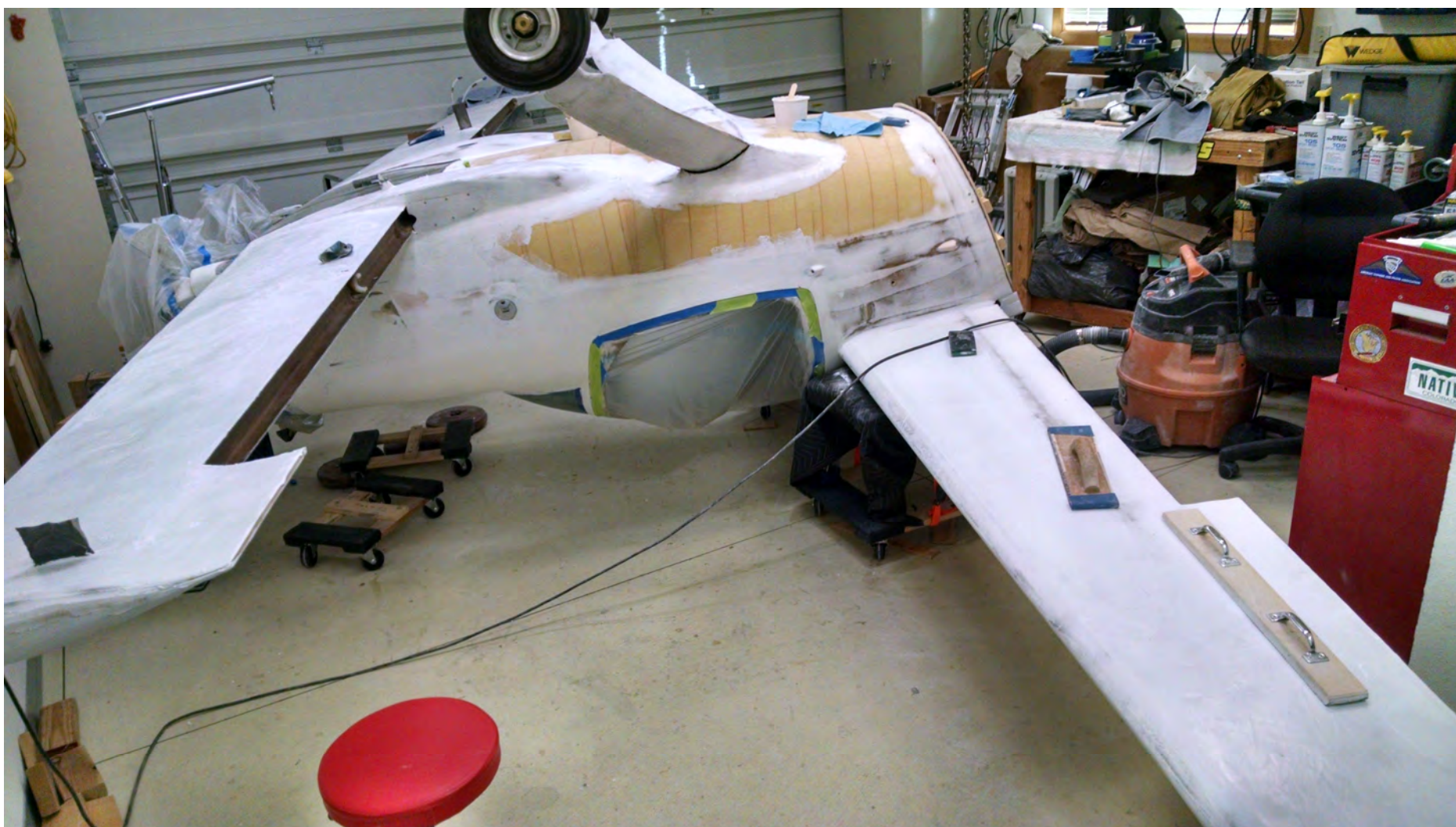
Fill and start contour sanding the bottom of the right main wing. October 2017
