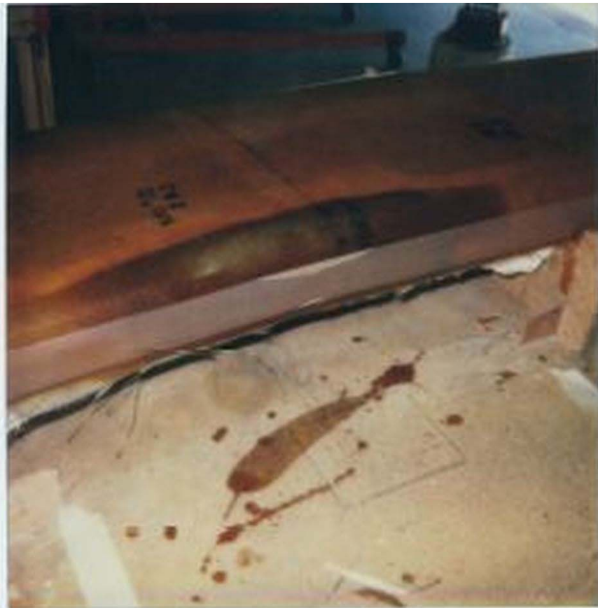
DETAIL Canard spar glassed & 6/15/85
