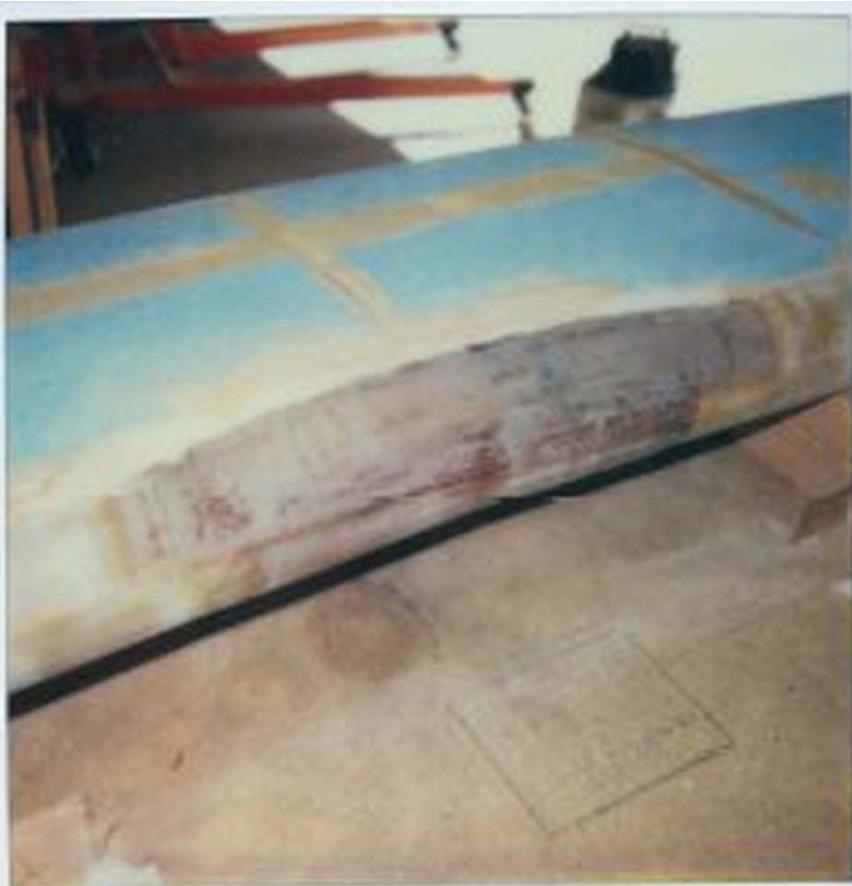
Detail bottom spar canard prepped for bottom skin 6/15/85
