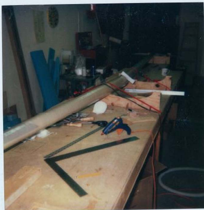
Canard spars being jugged and verified level 4/14/85
